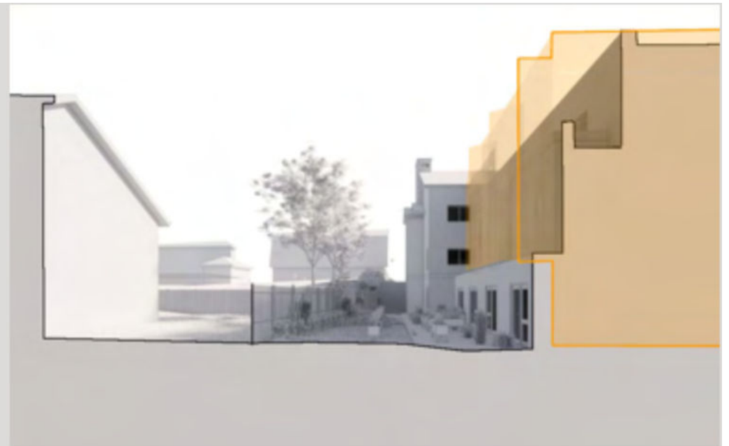
Comparative 3D Section view showing the refused scheme and proposed extension at the boundary shared with property No 6 Littlebrook.
